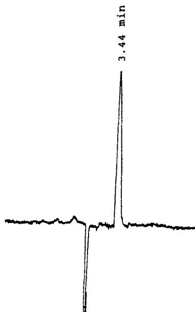
Figure 1 Electropherogram of lisinopril (SSS) and its RSS diastereoisomer. Conditions: fused silica capillary (72 cm (50 cm to detector), 50 \mu\text{m} i.d.); electrolyte: 25 mM tris- \text{PO}_4 , pH 9.55; applied voltage: 30 kV; 30 ^\circ\text{C} .
