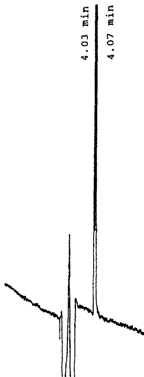
Figure 4 Electropherogram of lisinopril (SSS) and its RSS diastereoisomer using sodium cholate as the surfactant. Conditions: fused silica capillary (72 cm (50 cm to detector), 50 \mu\text{m} i.d.); electrolyte: 25 mM tris- \text{PO}_4 , 50 mM sodium cholate, pH 9.55; applied voltage: 30 kV; 30 ^\circ\text{C} .
